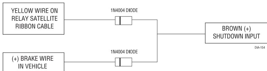
**IMPORTANT!** Once the interface is complete, attempt to remote start the vehicle with the door closed and the key in the ignition. The vehicle should not start. If it does, re-check the connections.
