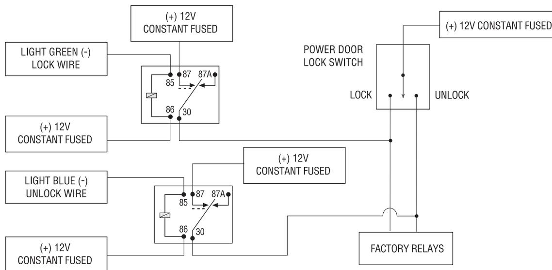
**type B: (-) pulses from the switch to the factory relays**
