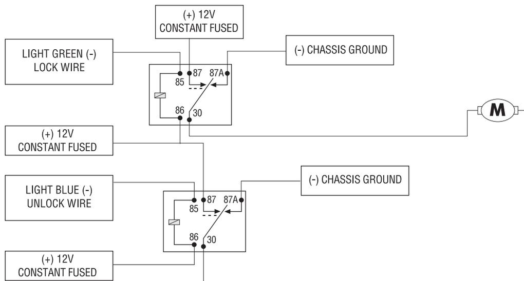
**IMPORTANT!** Do not connect the outputs of the alarm directly to the actuator!
