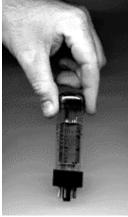
Make sure that the tube is oriented correctly when pulling it out or putting it back in. If you look at the end of the tube and the socket, you'll notice that the nine pins are arranged in an incomplete circle. Always make sure the pins are aligned correctly. Never force a tube into its socket.
