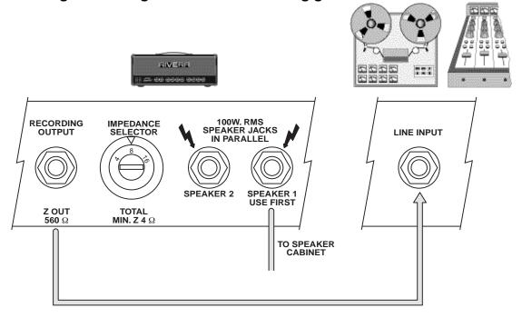
Using a shielded cord, connect the 's Recording Out to the line input or channel input of a mixer or recorder. (The signal comes from the amp's Preamp section, so all tone, distortion, and overdrive characteristics are included.) If you are not using the Effects Loop, you can use the Effects Loop Send jack instead of the Recording Out.
