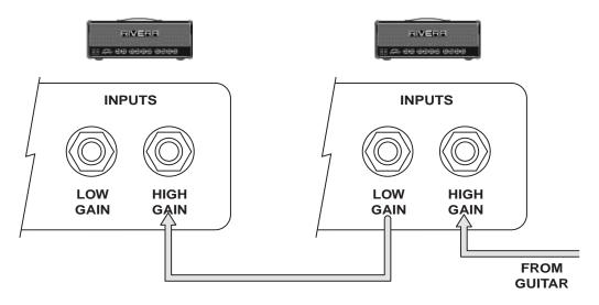
The Preamp and output amp sections, as well as all controls, function normally in this setup. Use a shielded cord. *Note:* Make sure that at least one speaker cabinet is connected to both amps unless you desire to use the Preamp sections only, in which case leave the Standby switch in the "Off" position.
