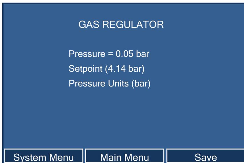
*Fig. 13: Gas Regulator screen (here: Corona Veo RS)*
