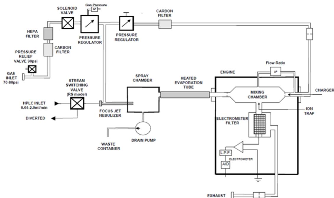
Fig. 29: Gas and aerosol flow paths inside the detector
