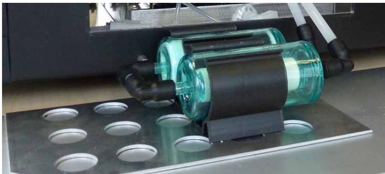
*Fig. 24: Replacing the gas filters*
