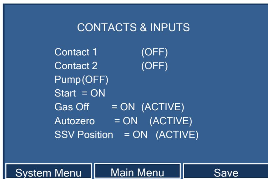
Fig. 15: Contacts & Inputs screen (here: Corona Veo RS)
