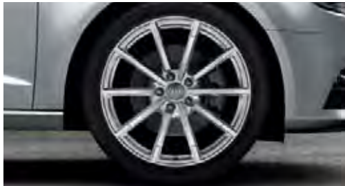
Audi exclusive cast aluminium wheels in 10-spoke design size 7.5 x 18 with 225/40 R 18 tyres 1 . From quattro GmbH
