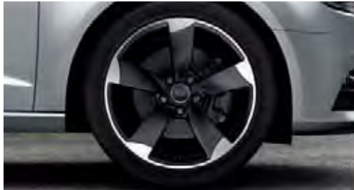
Audi exclusive cast aluminium wheels in 5-arm rotor design in matt black, gloss turned finish size 7.5 x 18 with 225/40 R 18 tyres 1 . From quattro GmbH
