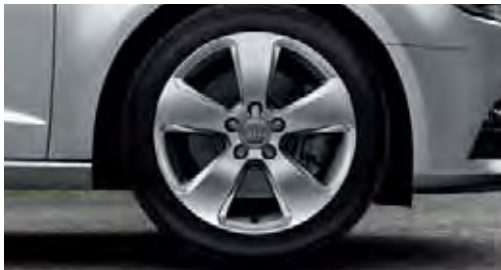
Cast aluminium winter wheels in 5-arm design size 6 J x 17 with 205/50 R 17 tyres 1 , permissible top speed 210 km/h, can be fitted with snow chains
