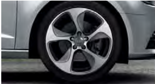
Cast aluminium wheels in 5-arm dynamic design anthracite, partly polished, size 7.5 x 18 with 225/40 R 18 tyres 1
