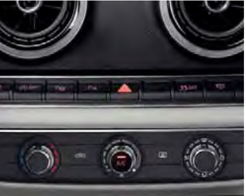
Manual air conditioning cools and heats up the vehicle passenger compartment, manually adjustable air distribution, manual recirculation mode, infinitely variable blower, 4 round vents in the dashboard that can be individually adjusted to provide directed or diffuse air flow, footwell vents at the front and rear, defroster nozzles for the windscreen and side windows, particulate filter
