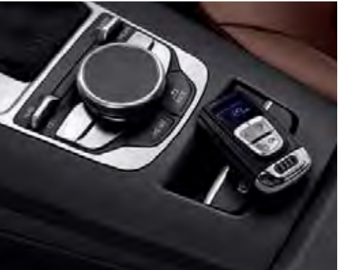
Auxiliary heating/ventilation The auxiliary heating warms up the interior and removes ice from the windows; the auxiliary ventilation system supplies fresh air and lowers the temperature on the interior; with timer and departure time programming (an intelligent control function for time and energy-efficient calculation of heating duration); separate radio-operated remote control with illuminated display
