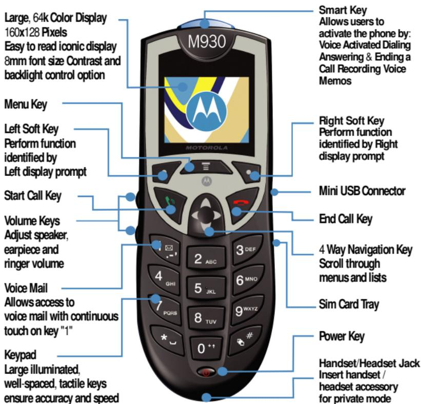
Figure 1. Basic diagram of the M930 In-Vehicle Phone.
