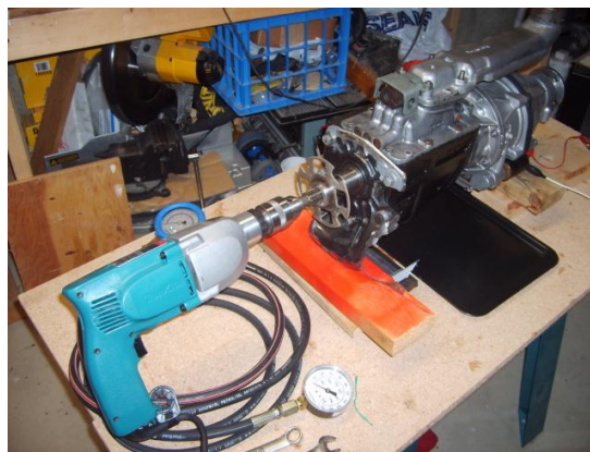
Figure 66 – RPM Testing Method
