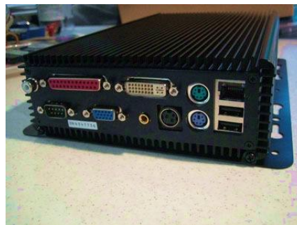
Figure 62 - Fins used to dissipate heat and keep elements out
