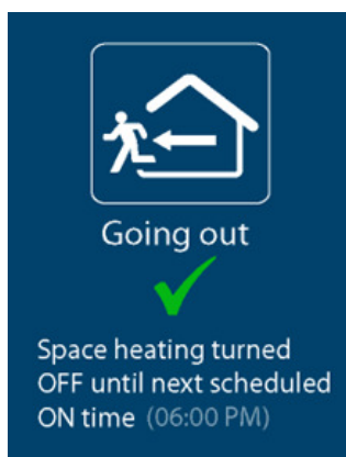
Figure 18: Going Out mode set. The heating will now remain switched off until the next scheduled on time
