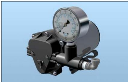
*Fig. D4: Connect pressure gauge to pump*
