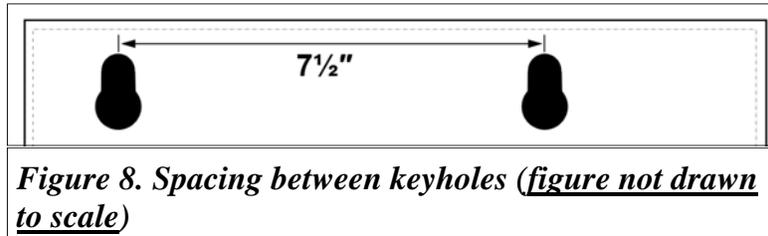
Install the screws (Figure 8) provided allowing for the thickness of the frame. (A pilot hole using a 1/16" drill bit is recommended for particle board side-walls.)
