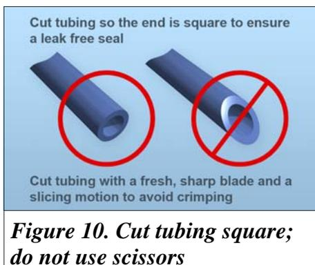
**Figure 10. Cut tubing square; do not use scissors**
