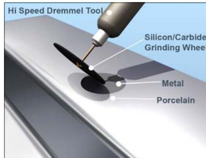
**Figure 3. Using a Dremmel Tool to remove porcelain**
