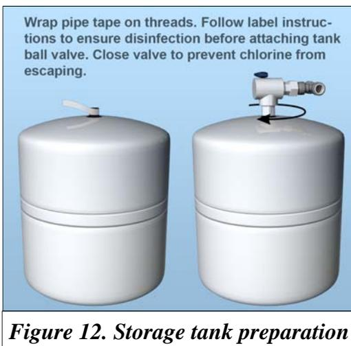
**Figure 12. Storage tank preparation**
