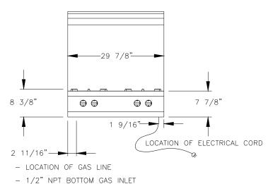
(MUST CONNECT TO NPT GAS SUPPLY LINE)
