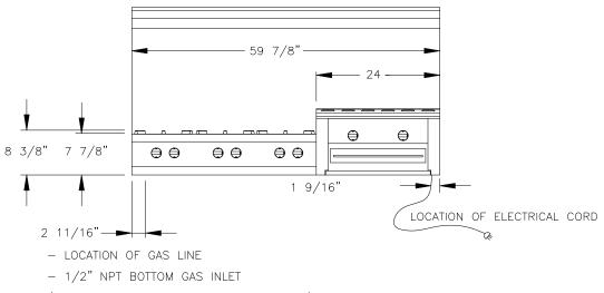
(MUST CONNECT TO NPT GAS SUPPLY LINE)
