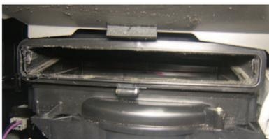
4. Install the filter element into the tray.
