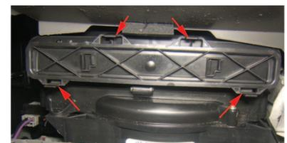
Parts can be found in the GM Dealers Parts Catalog under Group: 09.786, Description: Filter (Charcoal), Passenger Compartment Air; and Group: 09.786, Description: Cover, Passenger Compartment Air Filter Access Hole (Filter Tray).
