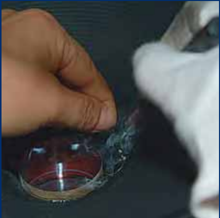
Voice coil / spider attachment on a 10-inch LF transducer.
