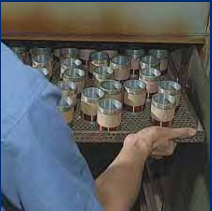
Coil baking. Nothin' sez lovin' like somethin' from the oven.
