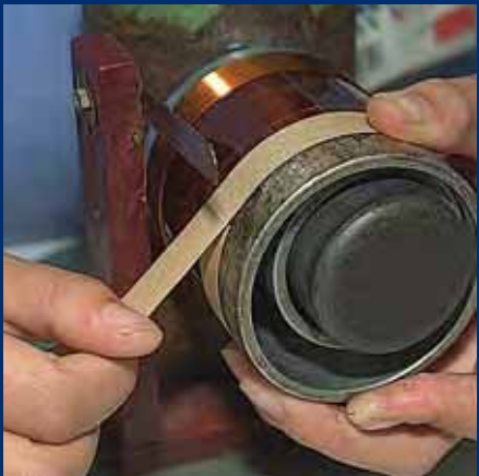
We wind over 100 different sizes of voice coils.
