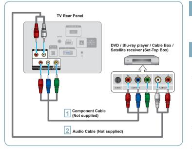
Connect a Component Cable between the COMPONENT IN [ Y,  $P_B$ ,  $P_R$ ] jacks on the TV and the COMPONENT [ Y,  $P_B$ ,  $P_R$ ] jacks on the DVD / Blu-ray player / Cable Box / Satellite receiver (Set-Top Box).
