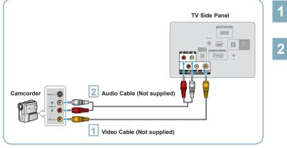
Connect a Video Cable between the COMPONENT IN / AV IN [VIDEO] jack on the TV and the VIDEO OUT jack on the camcorder.
