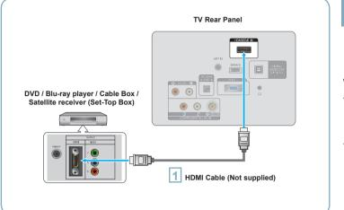
Connect an HDMI Cable between the HDMI (DVI) IN jack on the TV and the HDMI jack on the DVD Player or Cable Box / Satellite receiver (Set-Top Box).
