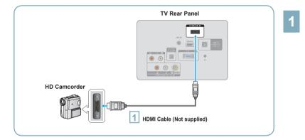
Connect an HDMI Cable between the HDMI (DVI) IN jack on the TV and the HDMI OUT jack on the camcorder.
