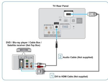
Connect a DVI to HDMI Cable or DVI-HDMI Adapter between the HDMI (DVI) IN jack on the TV and the DVI jack on the DVD / Blu-ray player / Cable Box / Satellite receiver (Set-Top Box).
