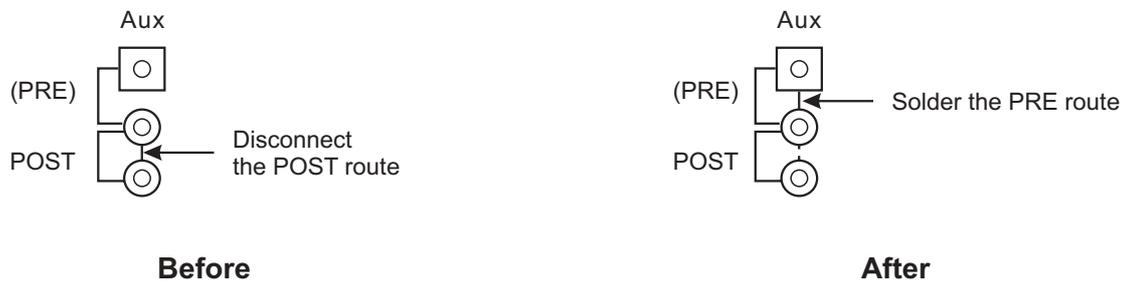
**Modification on mono and stereo channels**
