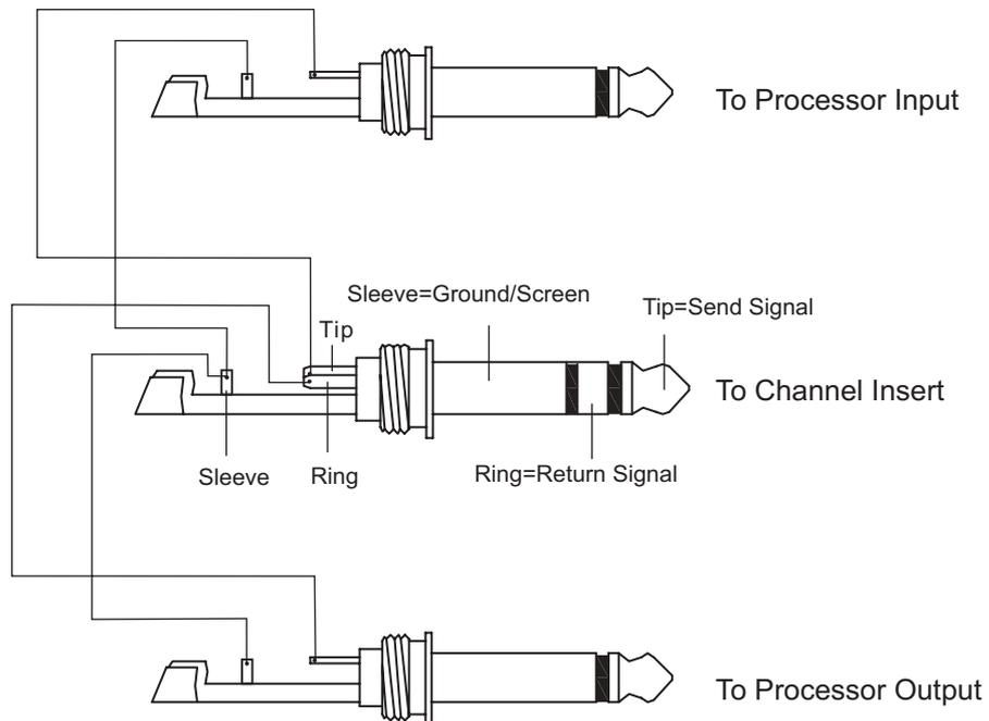
**Y-Stereo lead for insert Connection**
