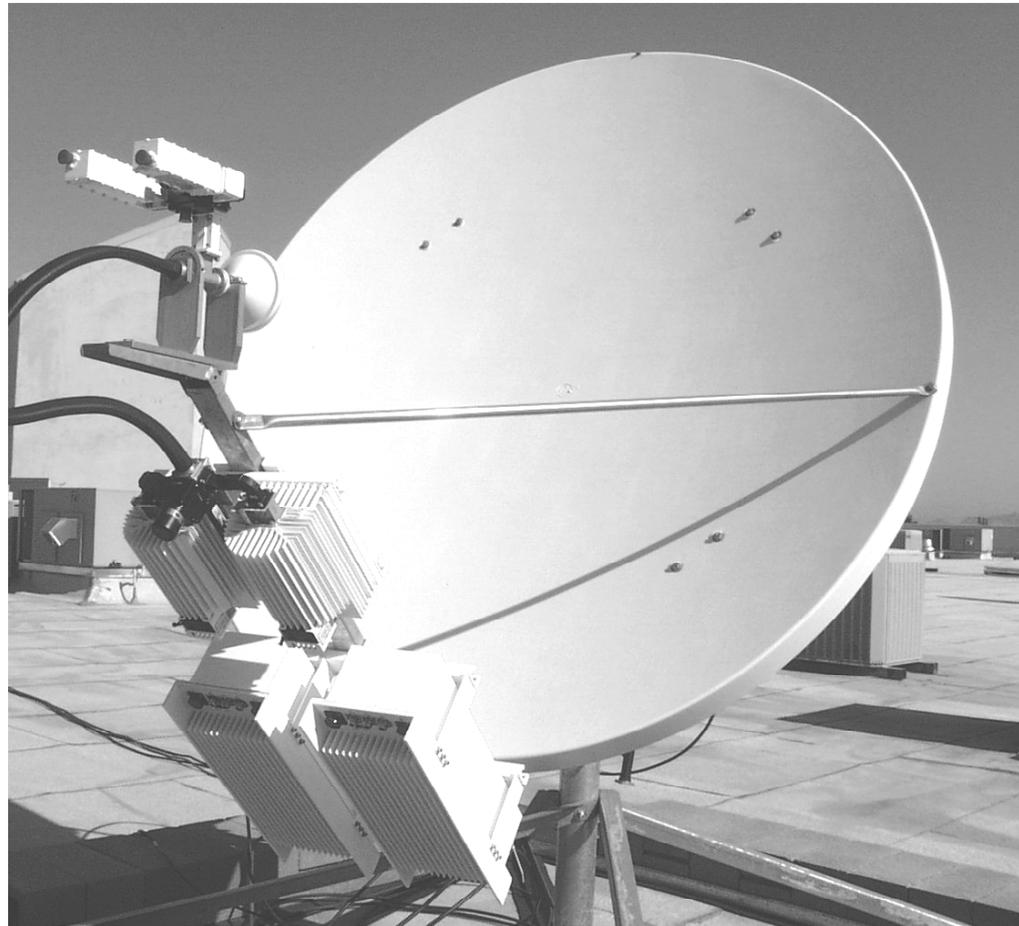
**Figure D-1. 1:1 System Installed on Spar Arm**
