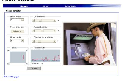
The VIP has an integrated video sensor which can detect changes in the signal. Such changes are due primarily to movements in the camera's field of view.
