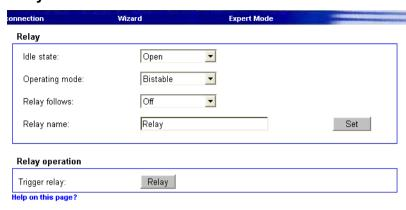
You can configure the switching behavior of the relay output. Relay action can be specified either as open switch (normally closed contact) or closed switch (normally open contact).
