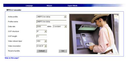
The data transmission parameters can be configured to suit the local operating environment (network architecture, bandwidth, data structures, etc.). Eight preconfigured profiles are provided in MPEG-2 mode, each reflecting different priorities and environments.
