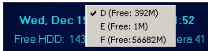
When the capacity of HDD is not enough or there has some mistakes while recording, system will pop up information to inform the failure of recording and the corresponding camera will stop recording.
