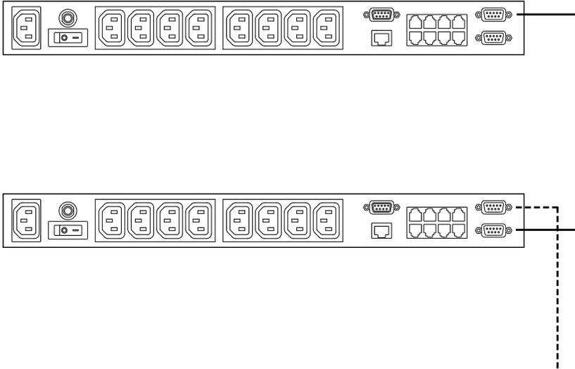
2. Power up the daisy chained PN9108U Stations in sequence starting with the highest level Station and working down. In each case, wait for the PN9108U's Station ID to be ascertained and displayed on the Station ID LED before powering on the next unit.
