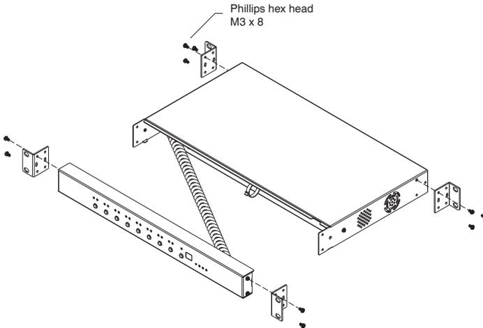
3. Position the device in the rack and align the holes in the mounting brackets with the hole in the rack.
