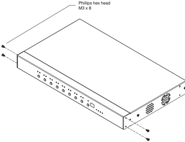
2. Use the screws you just removed, and the ones supplied with the rack mounting kit to screw the rack mounting brackets into both modules:
