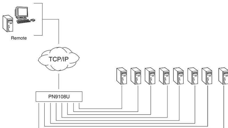
The power status of each outlet can be set individually, allowing users to establish on/off schedules for each device. Up to 15 additional PN9108U Stations can be daisy chained down from the original PN9108U, providing remote power management for up to 128 devices. Installation and operation is fast and easy: plugging cables into their appropriate ports and simple GUI management is all that is entailed.
