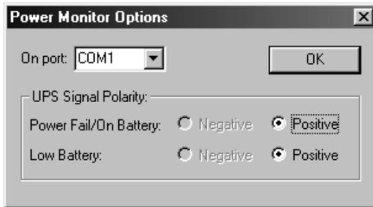
4. Open the list of COM ports, and select the COM port that the safe shutdown cable is connected to.
