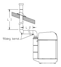
The flue temperature will be approximately 85 degrees C and should be kept at least 25 mm clear of any combustible surface.
