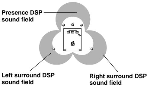
These programs use YAMAHA's tri-field DSP processing on each of the Dolby Digital or DTS signals for the front, left surround and right surround channels. This processing enables this unit to reproduce the immense sound field and surround expression of a Dolby Digital- or DTS-equipped movie theater without sacrificing the clear separation of all channels.
