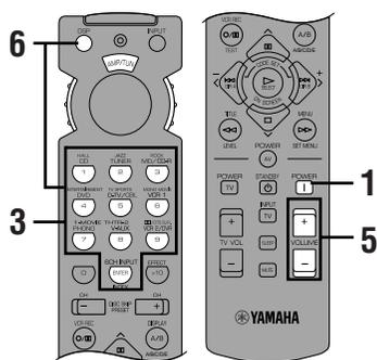
**3** Press **INPUT**  $\triangleleft/\triangleright$  repeatedly (or press one of the input selector buttons) to select the input source.
