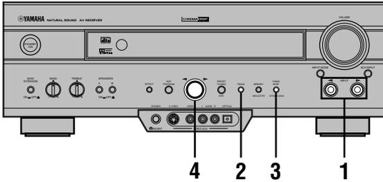
**1** Press INPUT </> to select TUNER as the input source.
