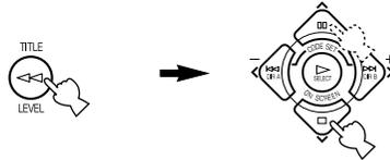
**5 Press </> repeatedly to adjust the output level of the currently selected speaker so that it becomes almost the same as that of the main speaker.**
