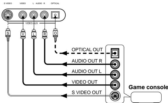
These jacks are used to connect any video input source such as a game console to this unit.
