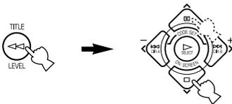
**3** Press **</>** to adjust the speaker output level.
