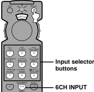
**1** Press INPUT regardless of the position of the selector dial. The indicator lights up for about 3 seconds.
