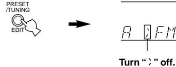
**4** Turn the multi jog knob to the right or left to tune in to the desired station manually.
