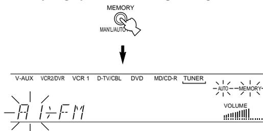
When automatic preset tuning is completed, the front panel display shows the frequency of the last preset station.
