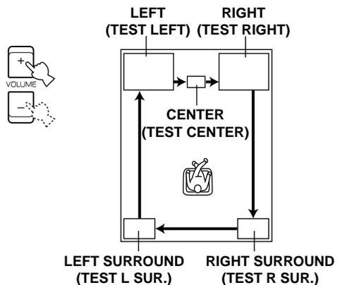
The state of the test tone output is also shown on the monitor by an image of the audio listening room. This is convenient for adjusting each speaker level.
