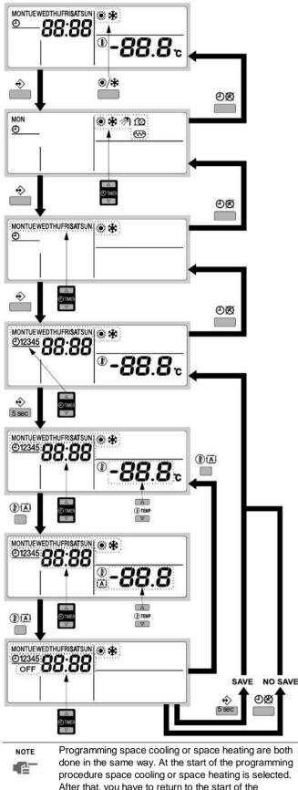
done in the same way. At the start of the programming procedure space cooling or space heating is selected. After that, you have to return to the start of the programming procedure to program the other operation mode.
