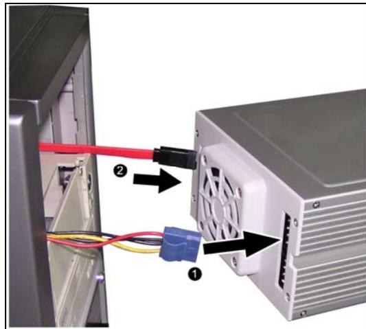
6. Insert the RAID box into the bay, and secure it in place with the screws provided. (If your case uses guide rails to install 5¼-inch devices, you can use them on the RAID box.)
