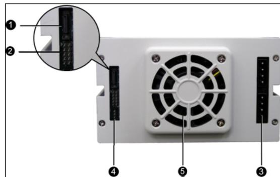
The **SATA cable** is the route used for reading and writing to the array.
