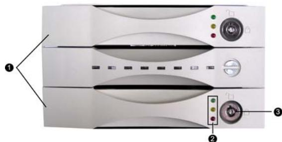
Each drive carrier can hold a one-inch high 3.5-inch form factor hard disk drive. This makes it easy to hot swap a drive in the event of a failure, without affecting the status of the remaining drives.
