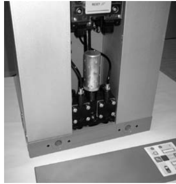
4. Dryer with front fascia panel removed.
