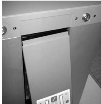
5. Re-fit front fascia panel by insertion of tongue into groove and pushing upwards and inwards.
