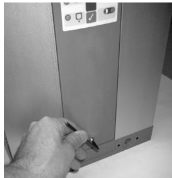
6. Replace single retaining screw.
