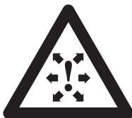
Caution: Risk of High Pressure
