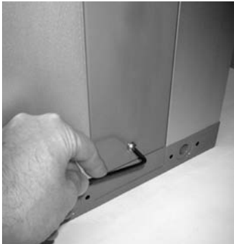
2. Remove single retaining screw.
