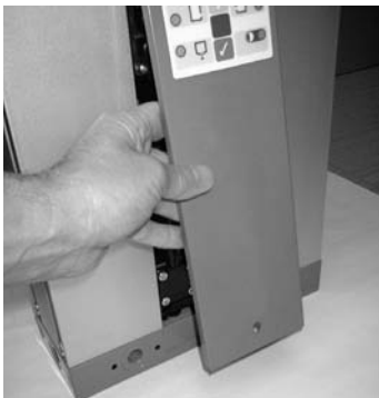
3. Remove front fascia panel by tilting outwards and downwards.
