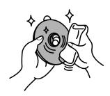
Clean the disc with water diluted with neutral detergent solution and wipe from inside to outside using dry cloth.
