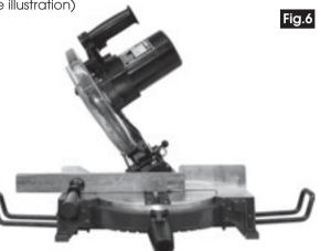
The  $45^{\circ}$  adjuster is factory set so that when the Head is tilted to its fullest extent the blade will cut  $45^{\circ}$  bevel.
