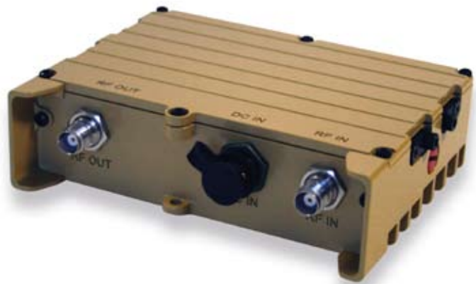
SOLO4 Robust Clip-on 1W Amplifier (L & S-Band)
