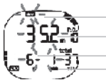
The DECO flag, current depth indication, decompression stop depth indication, and decompression stop time indication all flash, and an audible alarm sounds twice, for 3 seconds each time.
