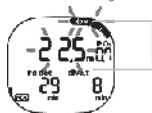
The SLOW flag (all graph) and current depth indication flash for 6 seconds, and an audible alarm sounds for 3 seconds.
