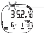
The DECO flag flashes for 15 seconds, and an audible alarm sounds twice, for 3 seconds each.
