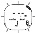
All indicated flags flash, and an audible warning sounds twice, for 3 sec. each time.
