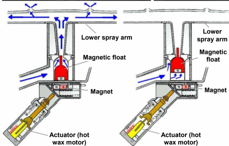
Models with water switches and *Top Rack Only* use water switches to divert water.
