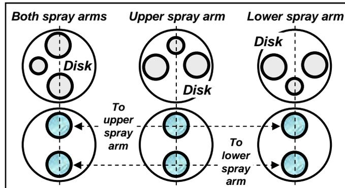
**HINT:** Models with water switches & *Top Rack Only* use water switches to divert water. Separate actuators aren't needed.
