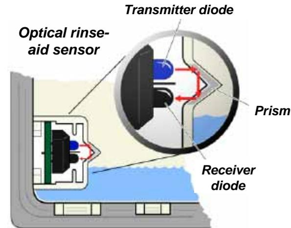
*When rinse-aid has run out, the optical receiver senses a strong light beam.*
