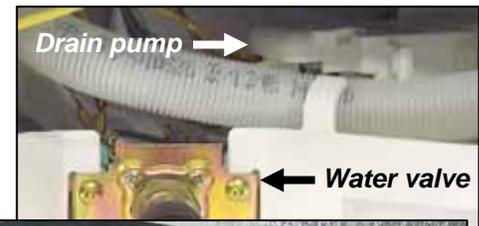
**NOTE:** Drain pumps in installations with Johnson Tees (in Washington State) must use stronger 4-vane pumps (# **184178**). Standard 9-vane drain pumps (# **167082**) are quieter and smoother than 4-vane pumps. Older pumps had 6-vanes.
