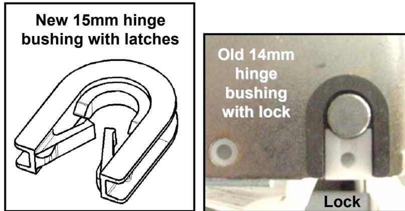
**NOTE:** New and old hinge levers and bushings can't be mixed and matched since new hinge levers have 15mm holes to fit new hinge bushings and old hinge levers had 14mm holes for old hinge bushings (and locks).
