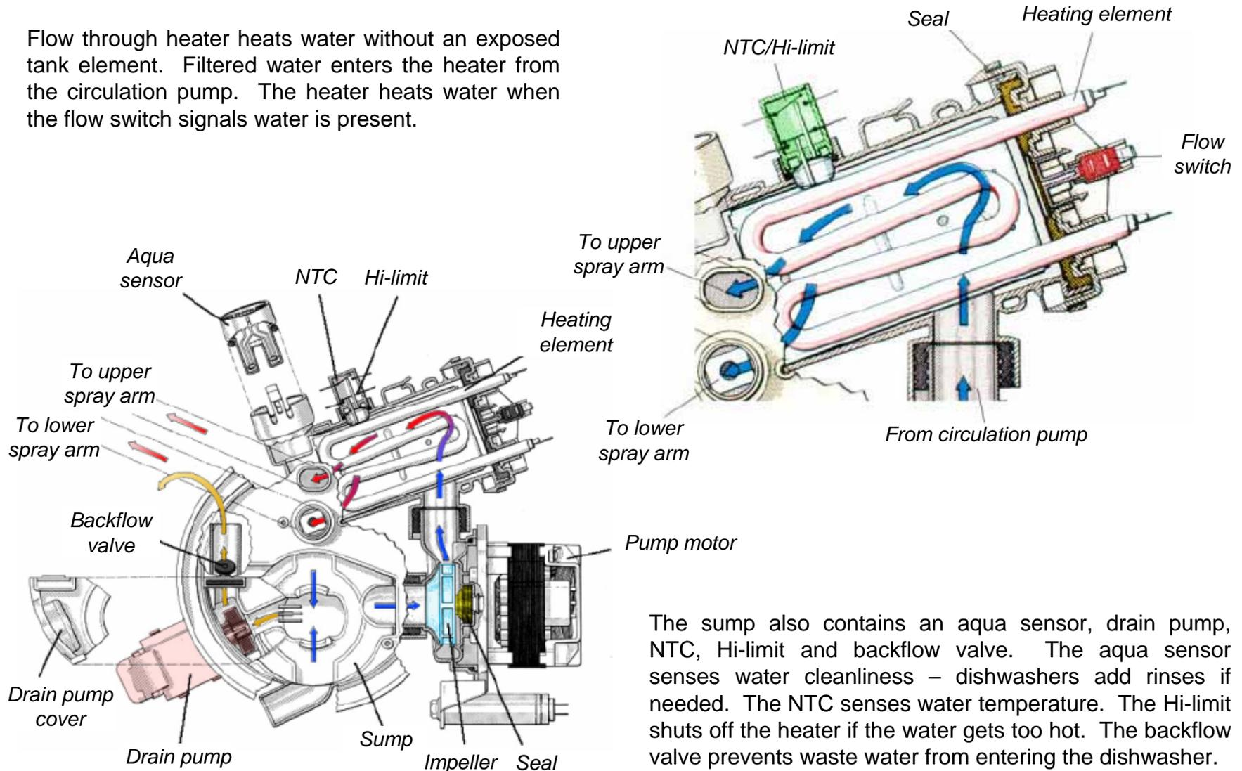
The sump also contains an aqua sensor, drain pump, NTC, Hi-limit and backflow valve. The aqua sensor senses water cleanliness – dishwashers add rinses if needed. The NTC senses water temperature. The Hi-limit shuts off the heater if the water gets too hot. The backflow valve prevents waste water from entering the dishwasher.
