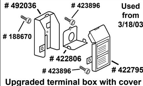
**NOTE:** Old terminal boxes built before 9/22/02 met UL standards – toe kicks were approved as terminal box covers. There's no need to change out old terminal boxes. Covers can't be added to these boxes since they don't have cover screw holes.
