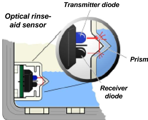
*With rinse-aid present, the optical receiver senses a diffused light beam.*
