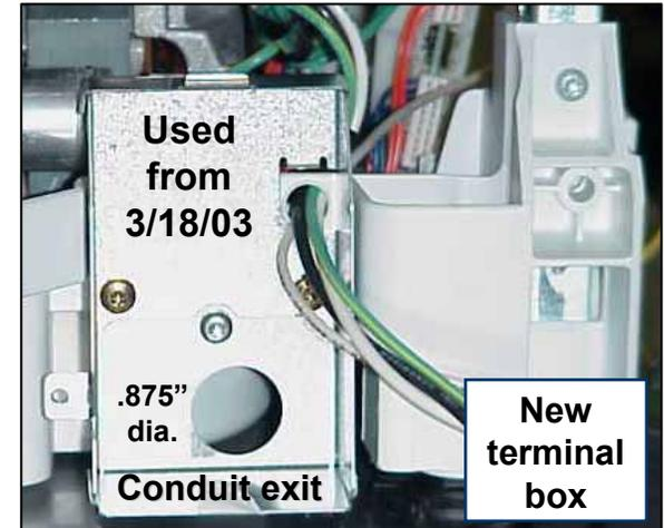
**TIP:** Proper installation requires strain relief on power cords/conduit! Use 3/8" or 1/2" fittings with .875" diameter.
