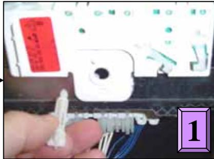
Inserting knob shaft into module
