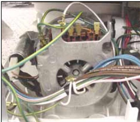
**HINT:** When replacing circulation pumps for softer bearing models (UC/11 & later), reusing existing front pump housings can save time by not changing hose clamps. If desired, order # **172272** hose clamps & replace entire pumps.
