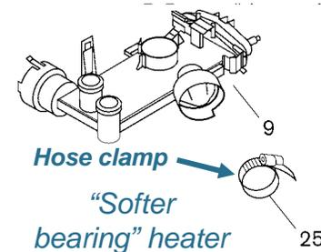
**HINT:** Heater assemblies contain NTC's, Hi-Limit's & flow switches (& aqua sensors where applicable). If heaters are replaced, these parts are replaced too.
