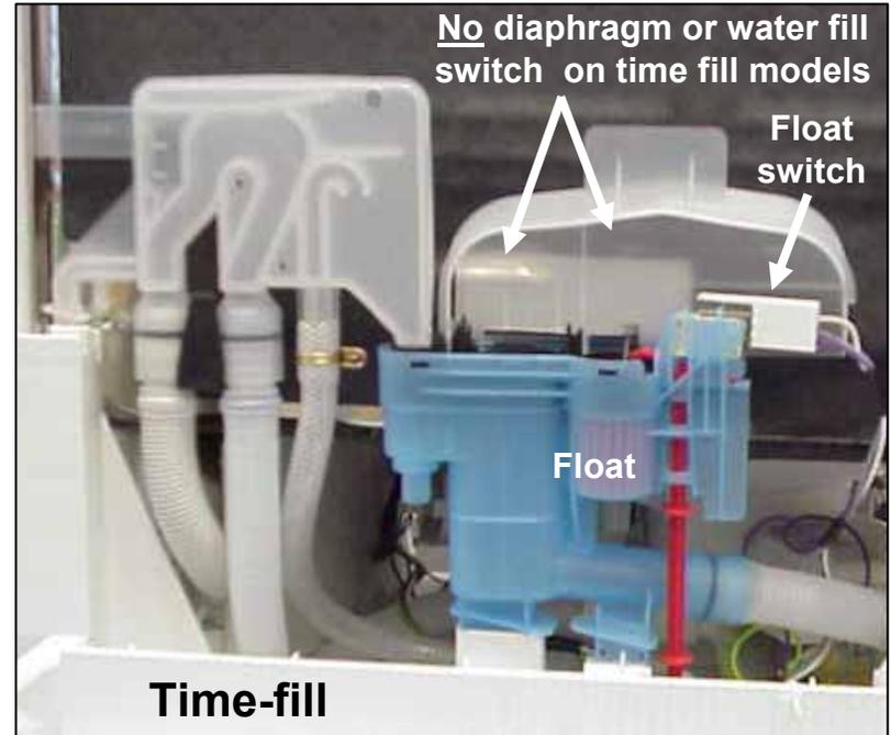
**HINT:** Most water fill assembly repairs involve replacing microswitches. Occasionally tank insulation or other debris can prevent the diaphragm switch lever from operating, allowing overfilling.
