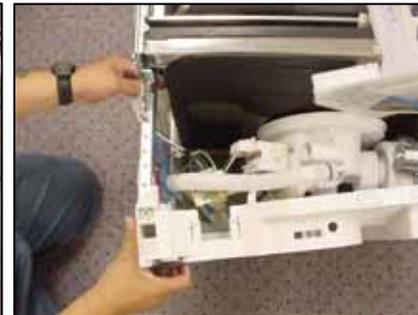
**Pulling base carefully from tank & sump**
