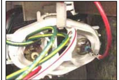
**HINT:** Because the flow switch only closes when water is flowing, the heater resistance can only be measured at the heater terminals (not at the control module).
