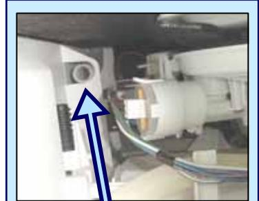
**HINT:** UC/12 (& later) model condensation tubes exit in the base behind the sump. There is no drain connection for these tubes.
