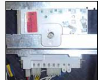
**HINT:** Knob shaft fits into knob only one way – line up knob with “cross” on knob shaft before attaching fascia panel to console.
