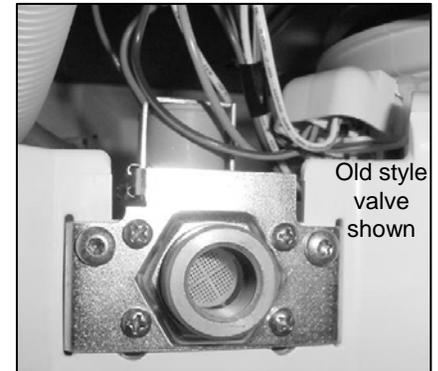
**CONNECTION HINTS:** Water connection 3/8" NPT female. Inlet water pressure range 5 - 120 psi (0.3 – 8.27 bars).
