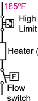
**NOTE:** Once its found one of these parts is faulty (from incoming current being 1.5 - 2A), check each part (once tank has been removed or blocked up) by measuring its resistance at its terminals:
