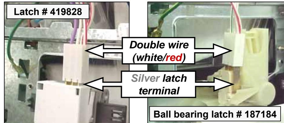
**CAUTION:** Operating dishwashers with miswired door latches will cause **irreversible** damage to control modules if doors have been closed and circulation pumps have started – modules must be replaced. Check door latch wiring whenever door latch terminals are changed or disconnected or when displays don't light up when dishwashers are turned on.
