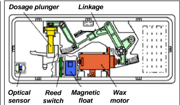
**NOTE:** The white plastic linkage opens the detergent dispenser door, then cocks in place to dispense rinse-aid when the wax motor operates again. After the 2nd operation, the linkage resets for the next wash.
