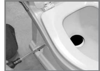
4. Turn screwdriver or socket wrench **counter-clockwise**. This will open flush ball and allow bowl contents to clear. After bowl is clear, turn screwdriver or socket wrench clockwise to return flush ball to original position.
