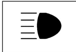
While the high beams are on, this light on the instrument panel cluster will also be lit.
