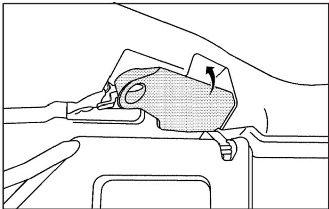
6. To unlock the release latches on the front of the roof panel, grasp each handle and pull it outward.
