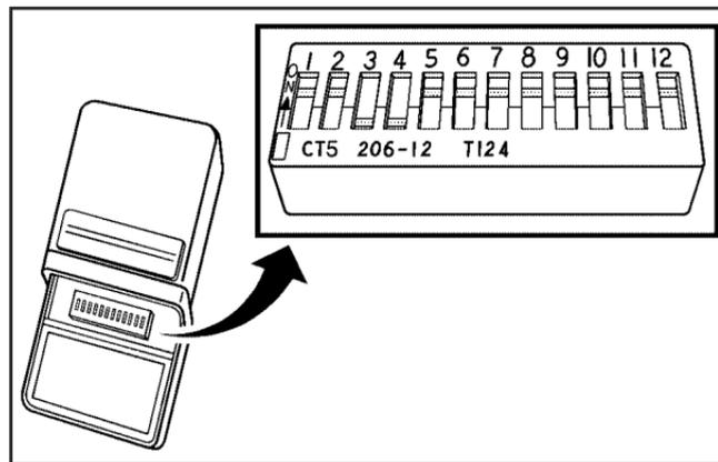
2. To verify that the garage door opener is a Fixed Code unit, remove the battery cover on the hand held transmitter supplied by the manufacturer of the garage door opener motor. If there are a row of dip switches similar to the graphic above, the garage door opener is a Fixed Code unit. If you do not see a row of dip switches, return to the previous section for Programming Universal Home Remote – Rolling Code.
