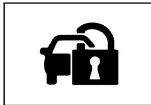
The security light flashes if a door is open and locked with the power door lock switch.
