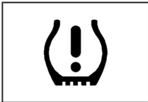
When a low tire pressure condition is detected, the TPMS illuminates the low tire pressure warning light, located in the instrument panel cluster.
