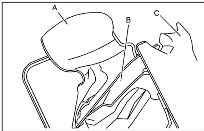
7. Lift the rear edge (B) of the convertible top to its full-up position by first raising the front edge (A).
