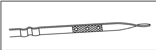
If the oil is below the cross-hatched area at the tip of the dipstick, add at least one quart/liter of the recommended oil. This section explains what kind of oil to use. For engine oil crankcase capacity, see *Capacities and Specifications* on page 5-110.
