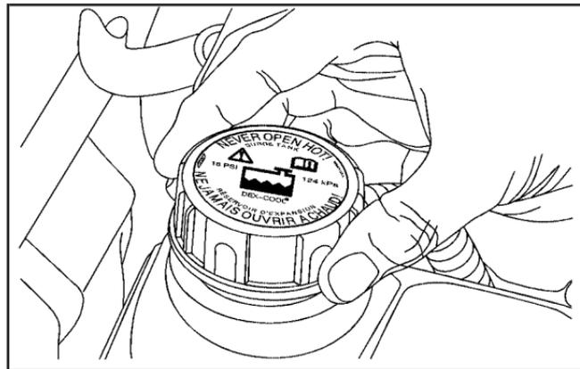
1. When the cooling system, including the coolant surge tank pressure cap and upper radiator hose, is no longer hot, remove the pressure cap. Turn the pressure cap slowly counterclockwise about one-quarter turn and then stop. If you hear a hiss, wait for that to stop. A hiss means there is still some pressure left.
