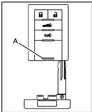
Press the button (A) near the bottom of the keyless access transmitter to remove the key. Never pull the key out without pressing the button.
