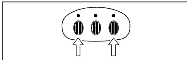
2. From inside the vehicle, press the two outside buttons at the same time for one to two seconds, and immediately release them.
