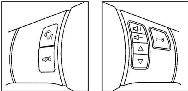
For vehicles with steering wheel controls, some audio controls can be adjusted at the steering wheel.
