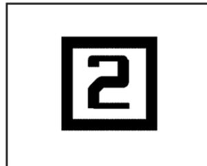
When using the Manual Paddle Shift feature while in S (Sport Mode), the current gear will be displayed in the Driver Information (DIC), or the Head-Up Display (HUD), if the vehicle has either of these features.
