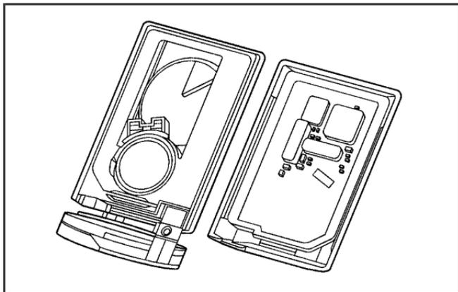
1. Separate the transmitter with a flat, thin object inserted into the slot on the side or back of the transmitter.
