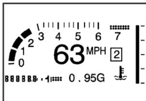
Track Mode 2 supports G-Force gages, boost gage w/ZR1, and minor gages with a linear tachometer.
