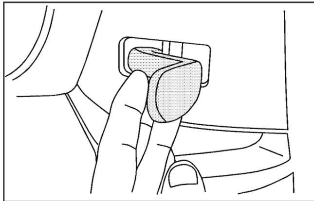
To tilt the wheel, hold the steering wheel and pull the lever toward you. Then move the wheel to a comfortable position and release the lever to lock the wheel in place.
