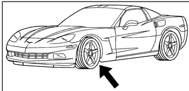
The front lifting points can be accessed from either side of your vehicle, behind the front tires.
