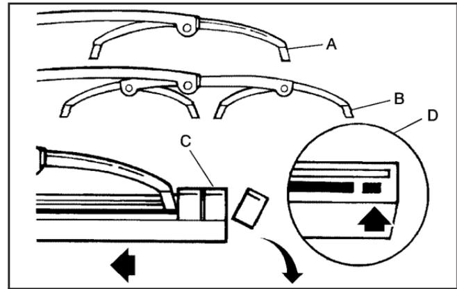
1. Slide the insert (D), notched end last, into the end with the two blade claws (A). Slide the insert all the way through the blade claws at the opposite end (B). The plastic caps (C) will be forced off as the insert is fully installed.
