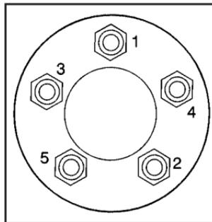
Tighten the wheel lug nuts firmly in a crisscross sequence as shown.
