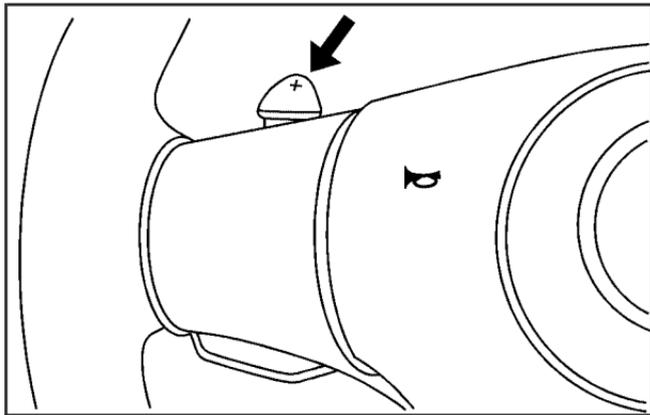
While in S (Sport Mode), push the paddle above the steering wheel spokes to up-shift to the next gear, or pull on the paddle behind the steering wheel spokes to down-shift to the next gear.
