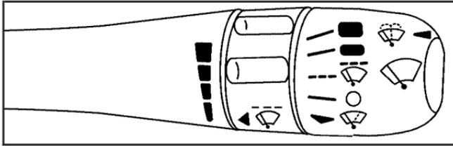
The windshield wiper lever is located on the right side of the steering column.
