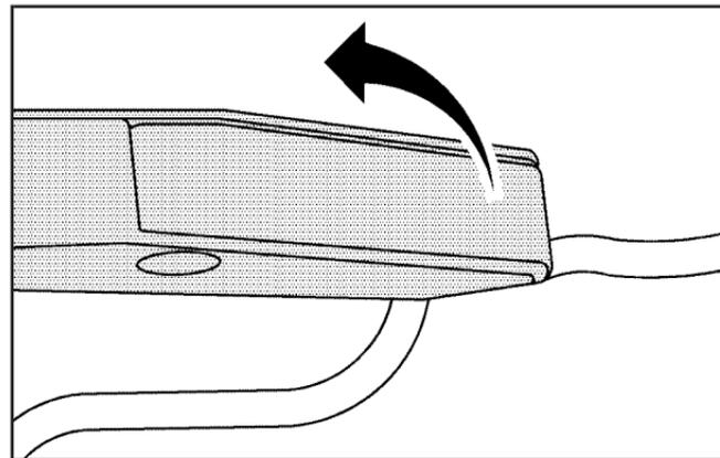
From inside the vehicle, use the door release handle located on the floor next to each seat. Pull the handle up to unlock and unlatch the door.
