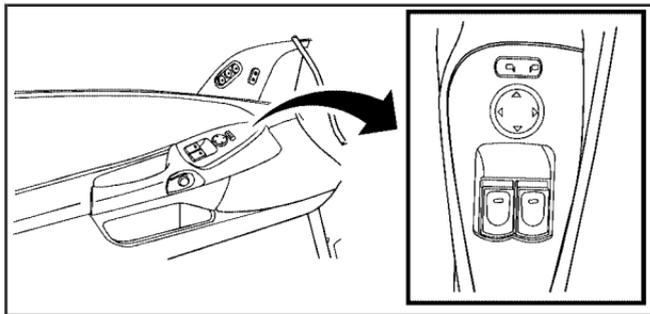
Controls for the outside power mirrors are located on the driver door.
