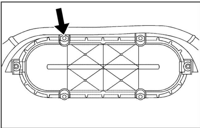
3. Remove the screws holding the filter element in place.
