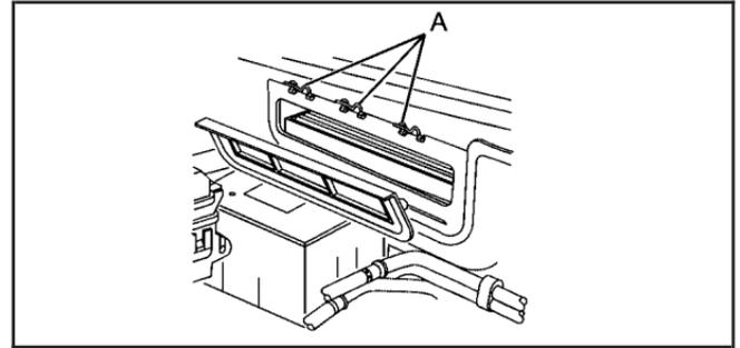
1. Remove the cover retainer clips (A) from the passenger compartment air filter cover.
