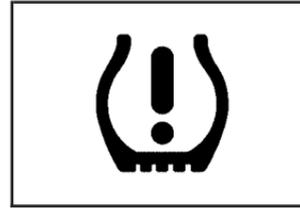
For vehicles with a tire pressure monitoring system, this light comes on briefly when the engine is started.
