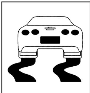
The Active Handling System light comes on briefly as the engine is started. If the light does not, have the vehicle serviced by your dealer/retailer. If the system is working normally the light goes off.
