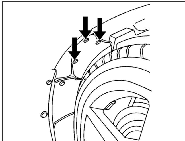
2. Remove the three outer fasteners to move the access panel back.
