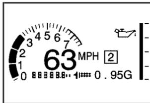
Track Mode 1 supports the G-Force gage and minor gages with a circular tachometer.
