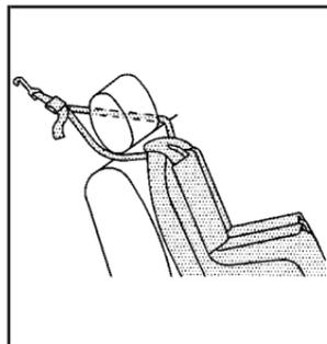
If the position you are using has a fixed headrest or head restraint and you are using a dual tether, route the tether around the headrest or head restraint.
