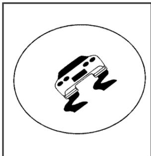
To turn the system off, press the ACTIVE HANDLING button on the console for five seconds. The system can be turned back on at any time by pressing the button. The DIC will display the appropriate message when the button is pushed.
