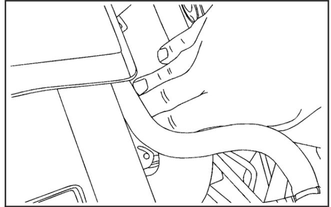
3. Fill the coolant surge tank with the proper DEX-COOL coolant mixture until the level inside stabilizes at the FULL COLD mark on the front of the surge tank.
