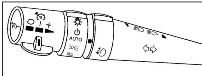
The exterior lamp control is located to the left of the steering wheel on the multifunction lever.
