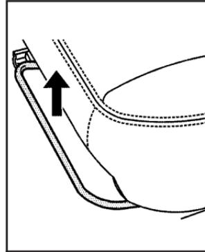
1. Lift the bar to unlock the seat.
