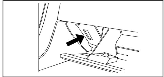
If moving the transmitter to different locations within the vehicle does not help, place the transmitter in the glove box transmitter pocket with the buttons facing to the right and then press the START button.
