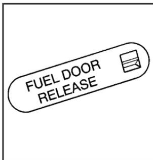
There is also a manual fuel door release tab. It is located against the upper trim in the rear compartment on the driver side of the vehicle. Pull the tab to release the fuel door.
