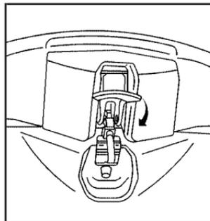
6. Turn the front release handles inward so that they latch to the closed position.
