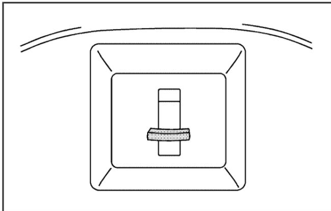
To fold a seatback forward, lift the latch located on top of the backside of the seat. The seatback locks when folded down.
