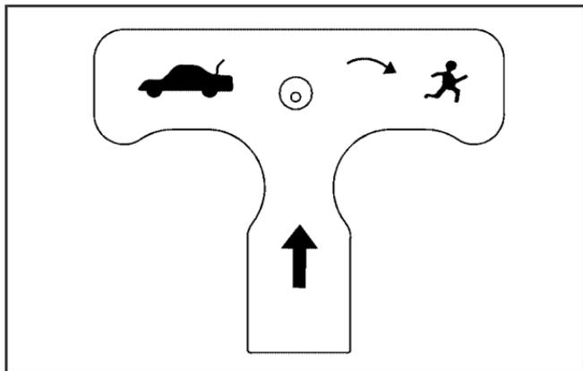
**Notice:** Do not use the emergency trunk release handle as a tie-down or anchor point when securing items in the trunk as it could damage the handle.
