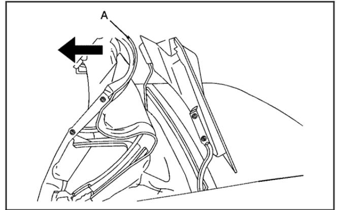
6. Pull the convertible top up by firmly gripping the front edge (A) near the center and applying a brisk upward and forward motion to get the top in the full-up position.
