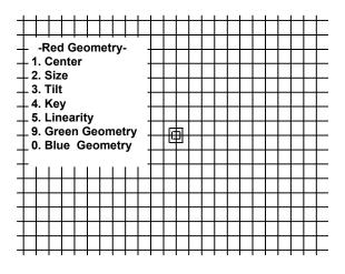
When Red Center adjustments are complete, press "2" to move directly to the next step.
