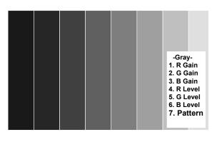
**NOTE:** When making gray scale adjustments with automated test equipment or color analyzers it is desirable to turn off the on screen menu instructions so that the color of the graphical instructions does not cause the instruments to register an incorrect reading. To turn the graphics off while making any of the gray scale gain or level adjustments press the "**ENTER**" button on the remote. Press it again to toggle the graphic back on.
