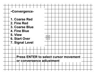
Better focus, in turn, deliver the most accurate convergence adjustments. For that reason, we recommend that, if possible, you lower the signal level to the greatest degree possible when converging the set.
