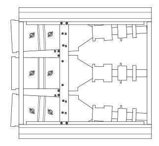
Refer to the diagram for the exact location of the three screws. The screws for the Red tube are marked on the diagram with an "R" and the screws for the Blue tube are marked with a "B". You may need to use a flashlight to locate the screw that connects the tube assembly to the floor pan.
