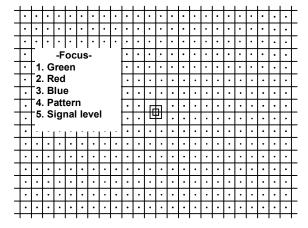
Use the left or right adjustment buttons on the remote (≺►), increase or decrease the signal level. When you have reached the desired signal level press "1" to display the Green Focus adjustment screen.
