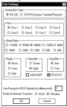
**NOTE:** The settings shown above represent the optimum RS-232 settings for loading to all Cresnet devices.
