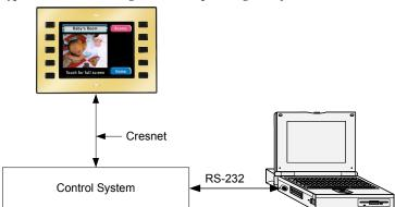
Typical Connection Diagram when Uploading a Project
