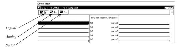
**NOTE:** Join numbers are expandable to 4000 digital & analog, 999 serial.
