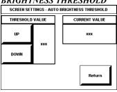
If the CURRENT VALUE has exceeded the THRESHOLD VALUE, the screen switches to high brightness. When the CURRENT VALUE is less than the THRESHOLD VALUE, the screen switches to low brightness.
