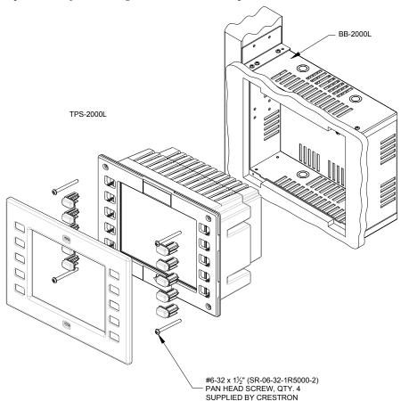
Exploded View for Mounting the TPS-2000L in the Optional BB-2000L Back Box
