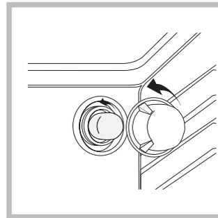
2. Remove the light bulb and replace it with a similar one: Wattage 25 W, cap E 14.
