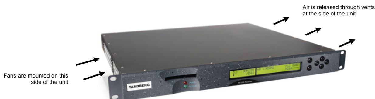
Figure 2.1: Air Flow Through the Equipment
