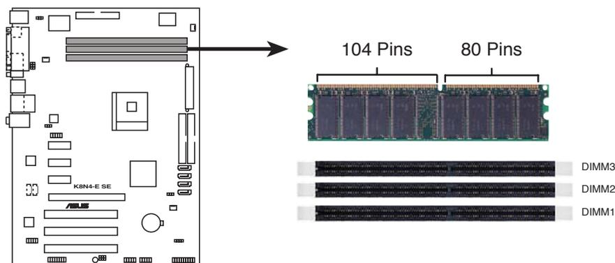
**K8N4-E SE 184-pin DDR DIMM sockets**
