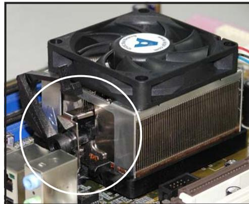
4. Push down the retention bracket lock on the retention mechanism to secure the heatsink and fan to the module base.
