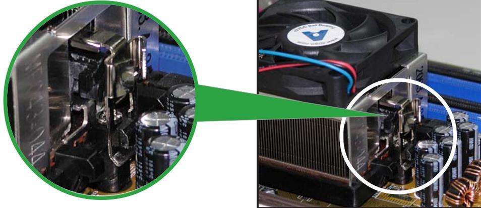
3. Align the other end of the retention bracket (near the retention bracket lock) to the retention module base. A clicking sound denotes that the retention bracket is in place.
