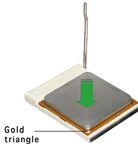
5. When the CPU is in place, push down the socket lever to secure the CPU. The lever clicks on the side tab to indicate that it is locked.
