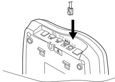
2. Plug the modular cord's other end into a modular telephone line jack.
