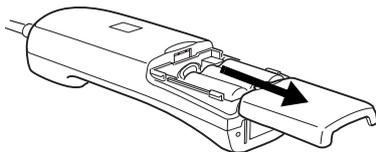
2. Lift the battery pack out of the compartment.
