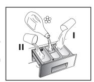
If liquid detergents are used, please insert the special container supplied into the compartment marked "II" in the detergent drawer. This ensures that the liquid detergent enters the drum at the right stage of the wash cycle.
