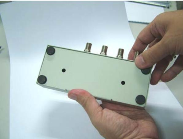
**Step 3** Press slightly on the back cover using the left hand thumb and slide the back cover using the right hand.
