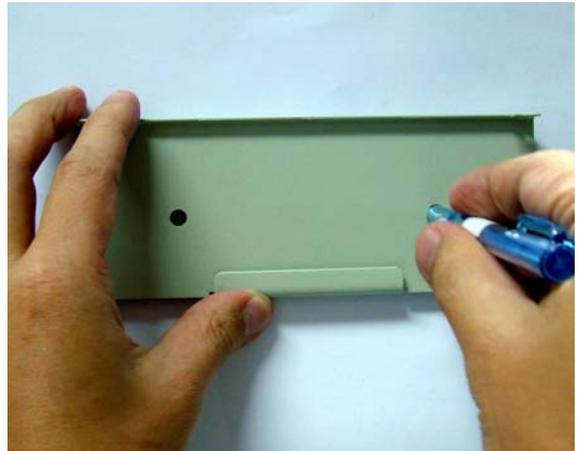
**Step 6** Prefer to drill a small hole on the location mark for easy mounting of the screws.
