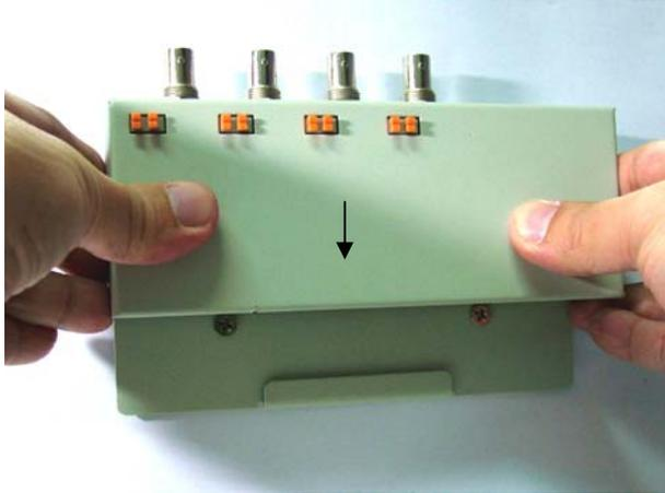
**Step 10** Use the thumb to press the orange terminal and insert the UTP cable.
