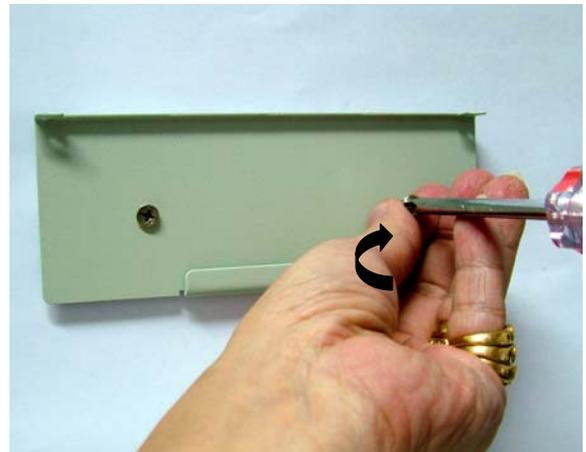
**Step 7** Slide the top cover onto the back cover with the slot on the top cover hook on the catch of the back cover.
