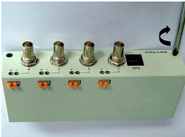
**Step 9** Strip the UTP cable with 5 mm copper exposed. Please take note on the polarity during installation.
