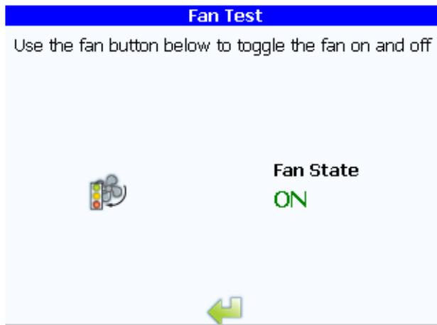
Figure 8-14 Fan test dialog box
