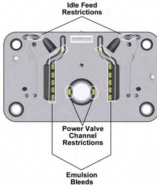
**3 Circuit Billet Metering Block (Front) Model 4500 Ultra HP DOMINATOR
