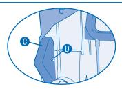
To replace either activity light unit **(**) (or to install/replace the batteries), remove screw **(**) and light unit from seat back.
