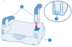
2. Assemble the backrest. Insert three posts ① on the headrest ⑥ into the backrest ⑥, as shown. Make certain the headrest locks securely into the backrest.
