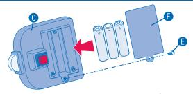
To install batteries in the activity light unit **(**0), remove screw **(**1) and battery door **(**2), install batteries as shown, then replace battery door and screw.
