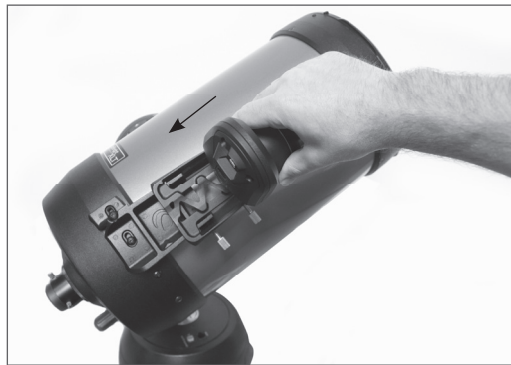
Installing large base (front to back)
