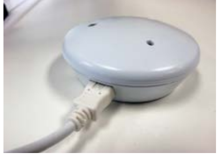
Figure 5. Charging cable installed. Note flat on cable is up.
