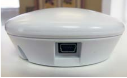
Figure 4. USB Mini-B style charging port on the TruStitch™ Controller.
