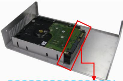
Place the hard disk face down and connector interface of hard disk in this direction.
