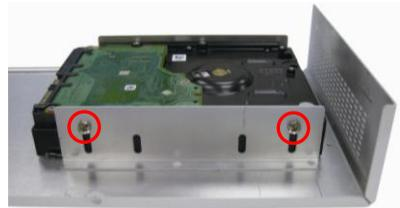
5. Hold the cover and connect the power cable and SATA cable to the hard disk. 6. And then, turn the cover over carefully.
