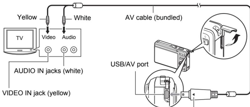
Making sure that the ► mark on the camera is aligned with the ◀ mark of the AV cable connector, connect the cable to the camera.
