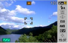
The image shows a camera viewfinder with a landscape scene. A semi-transparent Control Panel is overlaid on the right side of the frame. The panel contains various camera settings: a battery level indicator, a signal strength indicator, the number '123', a white balance icon, 'ISO', 'AWB', 'EV', and the time '15:37'. In the center of the image, there are four small icons representing focus, exposure, white balance, and zoom.                            |
