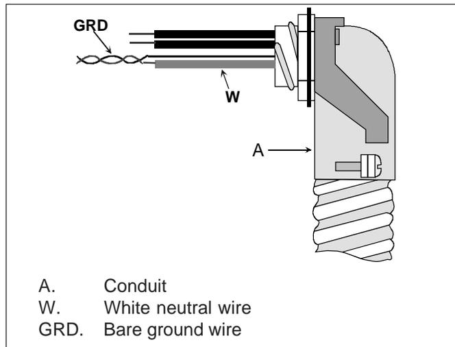
If oven is used in a mobile home or if local codes do not permit grounding through neutral, open connection and use grounding lead to ground unit in accordance with local codes. Connect neutral lead to branch circuit neutral conductor in usual manner.
