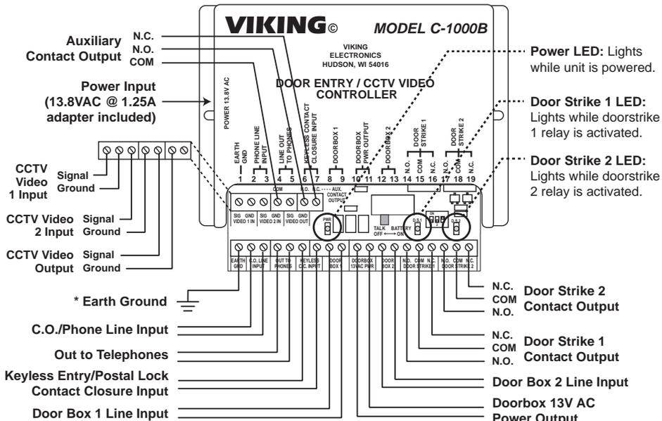
\* **Note:** To increase surge protection, fasten a wire from the screw terminal to Earth Ground (grounding rod, water pipe, etc.)
