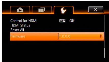
6. Touch the **[Firmware]** version number to display the firmware update confirmation screen. Touch **[OK]** to start the firmware update. After a short while, the firmware will be overwritten with the new version. (The update takes approximately 4 minutes.)
