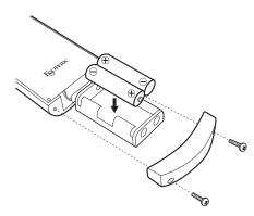
Remove the cover from the back of the remote control and insert two AA batteries with their  $\oplus/\bigcirc$  ends oriented as shown in the case. Replace the cover.
