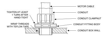
Figure 38: Water-Tight Seal Example
