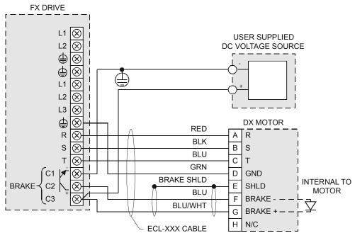
Figure 50: DX-490CB through DX-4120CB with Connectors
