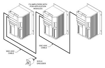
Figure 31: Encoder Cable Connections on a Multi-Axis Application
