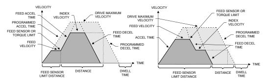
Figure 87: Velocity vs. Time Profile of a Registration Index
