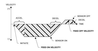
Figure 80: Feed On/Off Home Motion Profile
