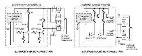
Figure 25: Pulse Mode Example of Sinking/Source Connections
