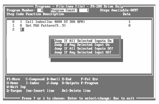
Figure 98: Jump on Input Pattern Commands Window
