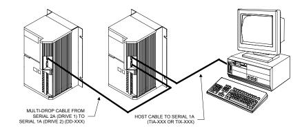
Figure 28: Multi-Drop Connections
