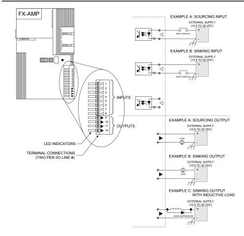
*Figure 34: Input/Output Connections*
