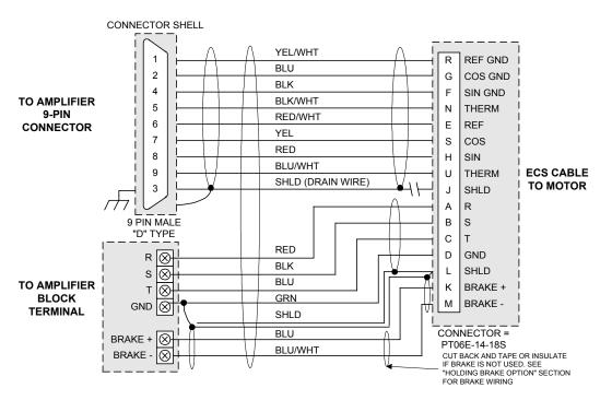
Figure 41: ECS Cable Wiring Diagram (FX-208 and DX-208C)
