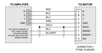
*Figure 42:* ECM Cable Wiring Diagram (FX-316 and DX-316C through FX-4120 and DX-4120C)
