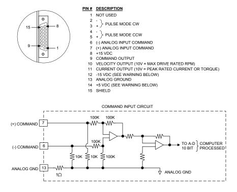
Figure 23: Command Connector Signals
