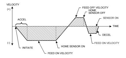
Figure 82: Feed On/Off/On Home Motion Profile
