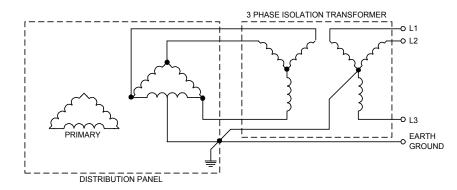
*Figure 15: Phase Delta/Delta Distribution to a Three-Phase WYE/WYE Isolation Transformer*
