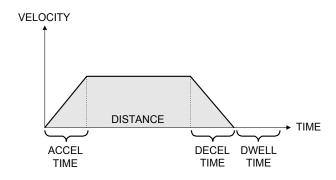
*Figure 3: Indexing Mode Diagram*
