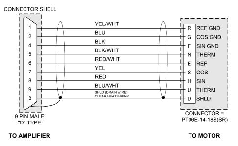
Figure 40: ECF Cable Wiring Diagram, FX-316 through FX-4120
