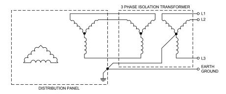
*Figure 16:* Three-Phase Delta/WYE Distribution to a Three-Phase WYE/WYE Isolation Transformer
