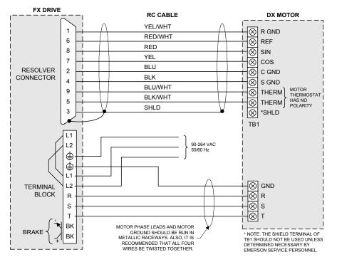
Figure 35: Motor Wiring, DX-316 through DX-455
