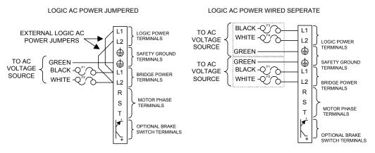
Figure 9: Fuse Wiring
