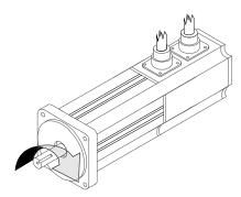
*Figure 65: Clockwise (+) rotation of the motor*
