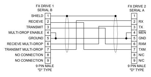
Figure 32: DD-XXX Wiring Diagram (Multi-Drop Cable)
