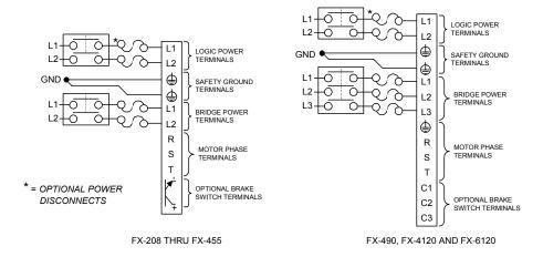
Figure 10: External Disconnect Example (FX-208 through FX-6120)
