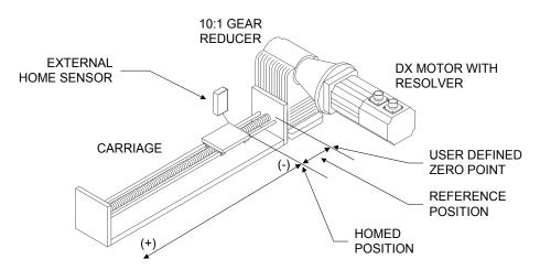
Figure 75: Home Cycle Example of Feed On/Off/Offset
