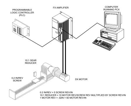
Figure 61: FX Drive System Example
