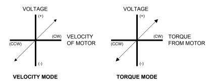
Figure 21: Analog Velocity/Analog Torque Modes
