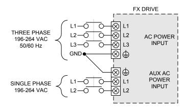
Figure 12: Typical Three-Phase Connection (FX-6200 through FX-8400)
