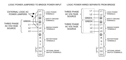
Figure 11: Typical Three-Phase 230VAC (FX-490 through FX-6120)
