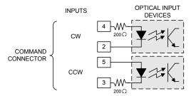
Figure 26: Command Connector Circuit Pulse Command Signals
