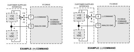
Figure 24: Customer Supplied Interface to the Command Connector
