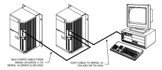
Figure 6: Serial Communication Multi-Drop Setup Example
