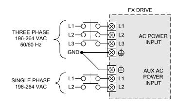
Figure 1: External Disconnect Example (FX-6200 through FX-4800)
