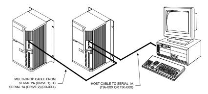
Figure 59: Establishing Serial Communications in a Multi-drop system
