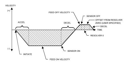
Figure 81: Feed On/Off/Offset Home Motion Profile
