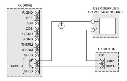
Figure 46: DX-490WB through DX-6120WB Motors without Connectors
