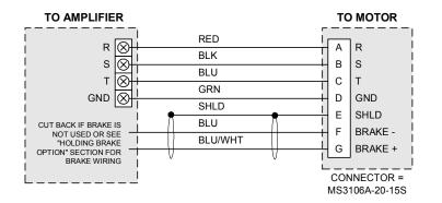
*Figure 43:* ECL Cable Wiring Diagram (FX-490 and DX-490C through FX4120 and DX-4120C)
