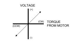
Figure 5: Analog Torque Mode Diagram
