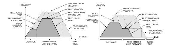
Figure 86: Velocity vs. Time Profile of a Feed Sensor Index
