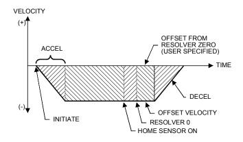
Figure 79: Feed On / Offset Home Motion Profile
