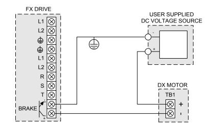
Figure 45: DX-316WB through DX-455WB Motors without Connectors
