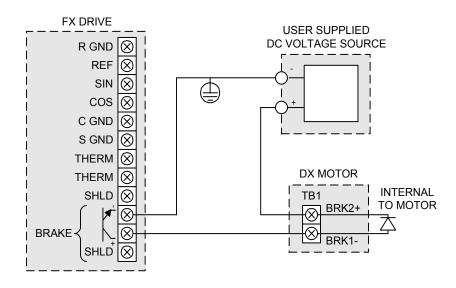
Figure 47: DXM-6200WB through DXM-8400WB Motors without Connectors
