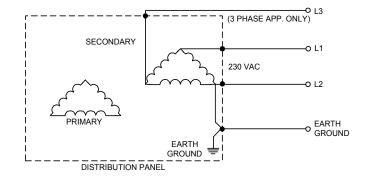
Figure 14: Earth Grounded Delta Distribution Transformer
