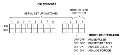
Figure 20: FX Drive Front Panel DIP Switches/Mode Selection
