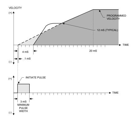
Figure 70: Velocity vs. Time Profile of High Speed Inputs
