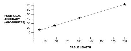
Figure 30: Positional Accuracy vs. Cable Length
