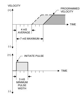
Figure 69: Velocity vs. Time Graph Showing Input Response Time
