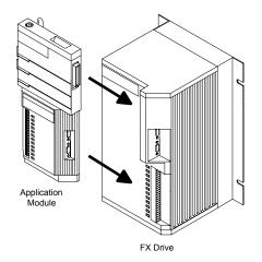
Figure 8: Application Module (PCM) Attaches to FX Drive
