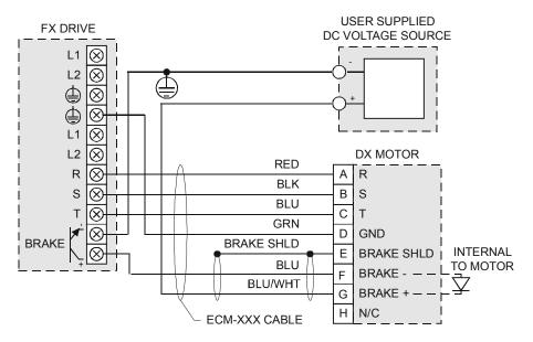
Figure 49: DX-316CB through DX-455CB Motors with Connectors
