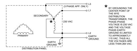
Figure 13: Earth Ground WYE Distribution Transformer
