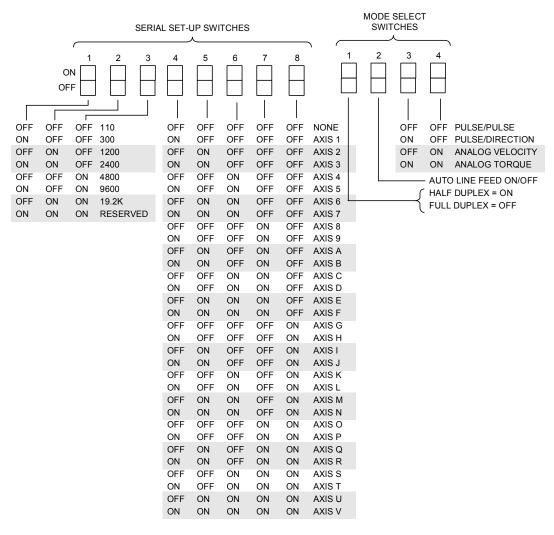
Figure 29: FX Drive Front Panel DIP Switches
