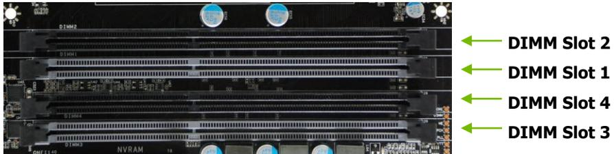
Use the following procedure to install memory DIMMs. Note that there is only one gap near the center of the DIMM slot. This slot matches the slot on the memory DIMM to ensure the component is installed properly.
